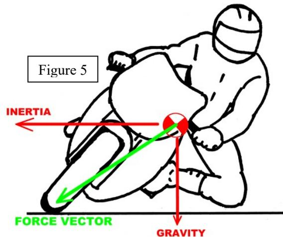
Because the rider cannot change his weight or the bikes weight, the force of gravity pushing down on the tire is always one (1) g thus the resulting friction will remain constant. The only thing the rider can change is the force of inertia by changing speed or radius.
