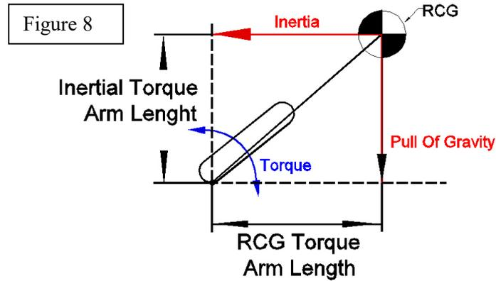
force is perpendicular to the gravitational pull on the RCG. The vertical distance between the RCG and the tire contact patch can be thought of as the vertical inertial torque arm. The inertial force times the torque length will develop a torque around the contact patch and try to pull the bike back up.
